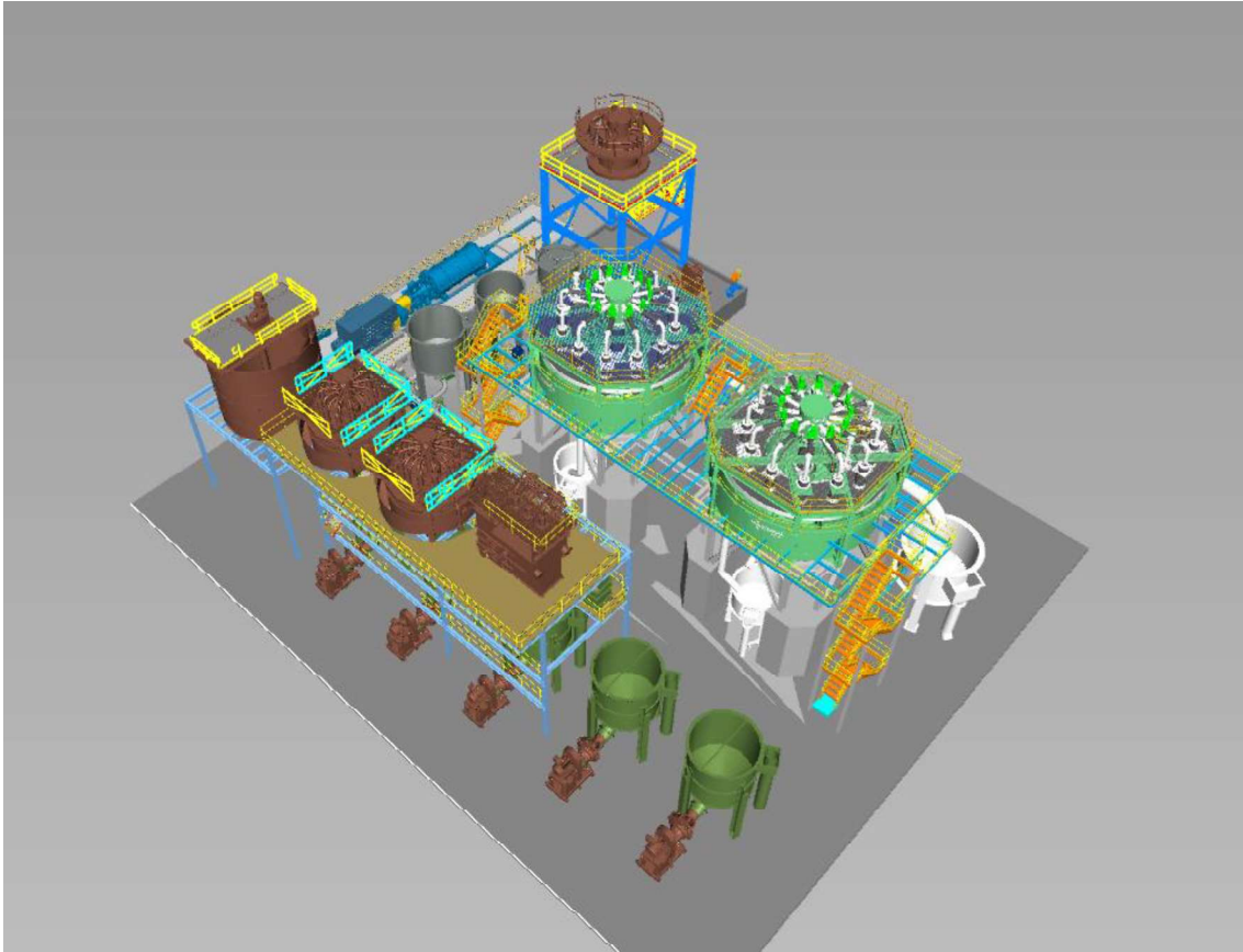
Figure 5: Plant Layout - Jameson Concentrator
