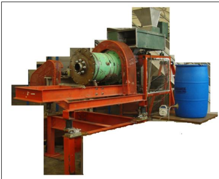
Figure 5: The pilot ball mill with interchangeable discharge end (overflow and grate discharge).
