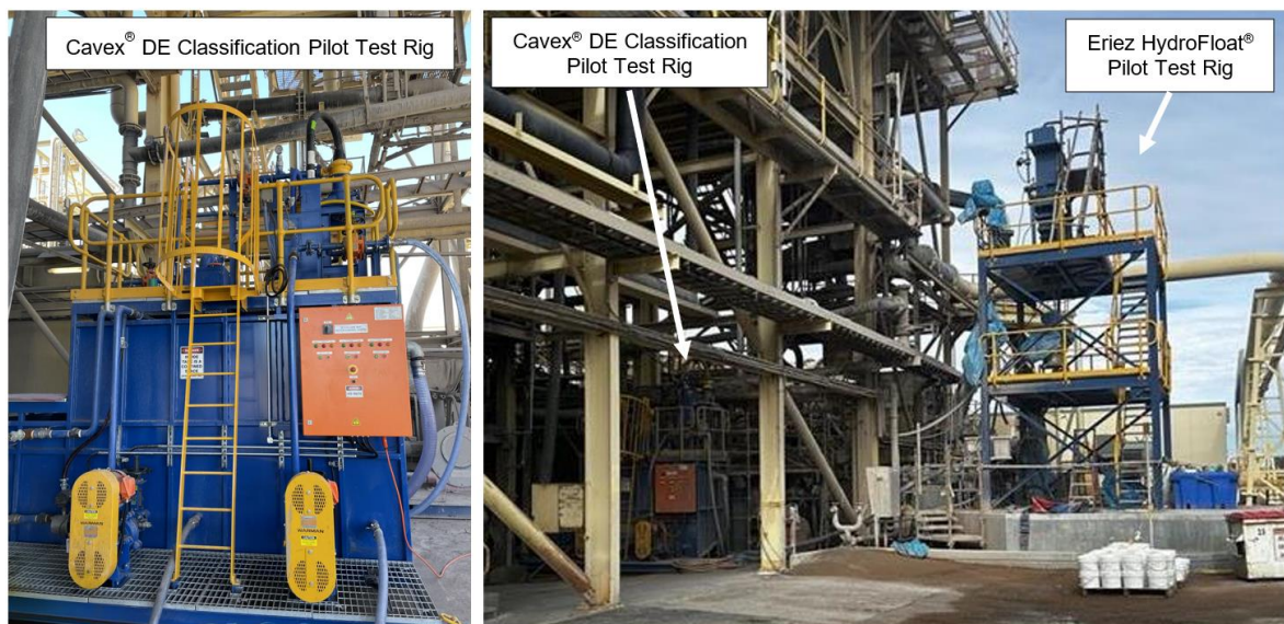
FIG 11 – Cavex ® DE hydrocyclone and Eriez HydroFloat ® Pilot test rigs.
