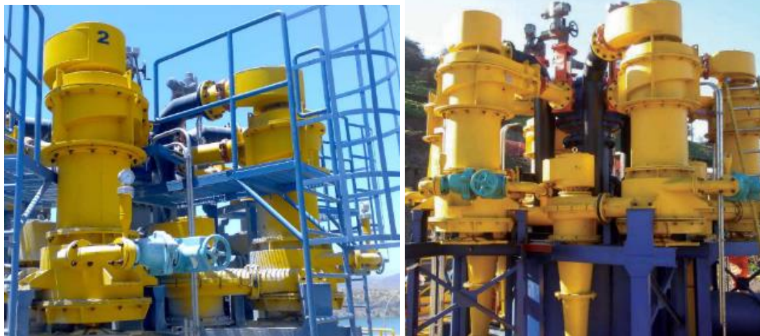
FIG 12 – Cavex® DE hydrocyclone cluster installation examples (bottom) and in a tailings facility in South America (top).
