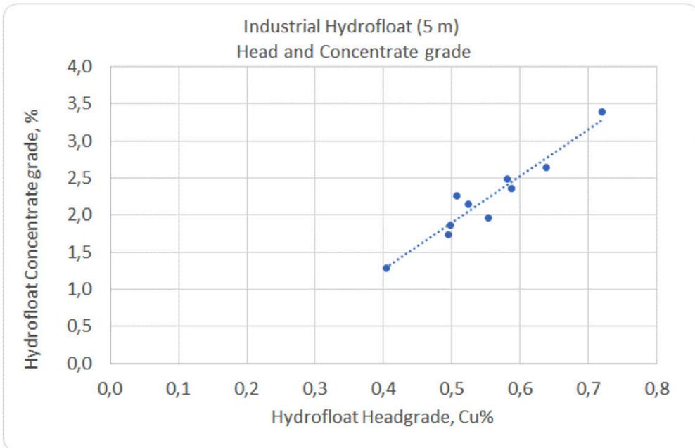
**Figure 9: Monthly average HydroFloat feed and concentrate grades.**
