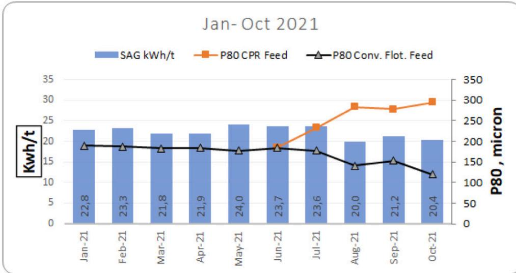
Figure 6: SAG kWh/t, P80 Feed to CPR and P80 Feed to Conventional Flotation, Jan. to Oct. 2021.
