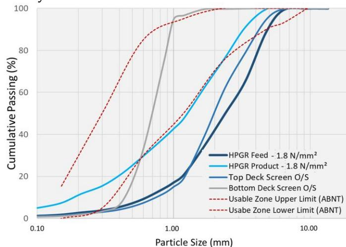
Figure 9. Survey 2 size distributions and limits for use as sand for concrete.
