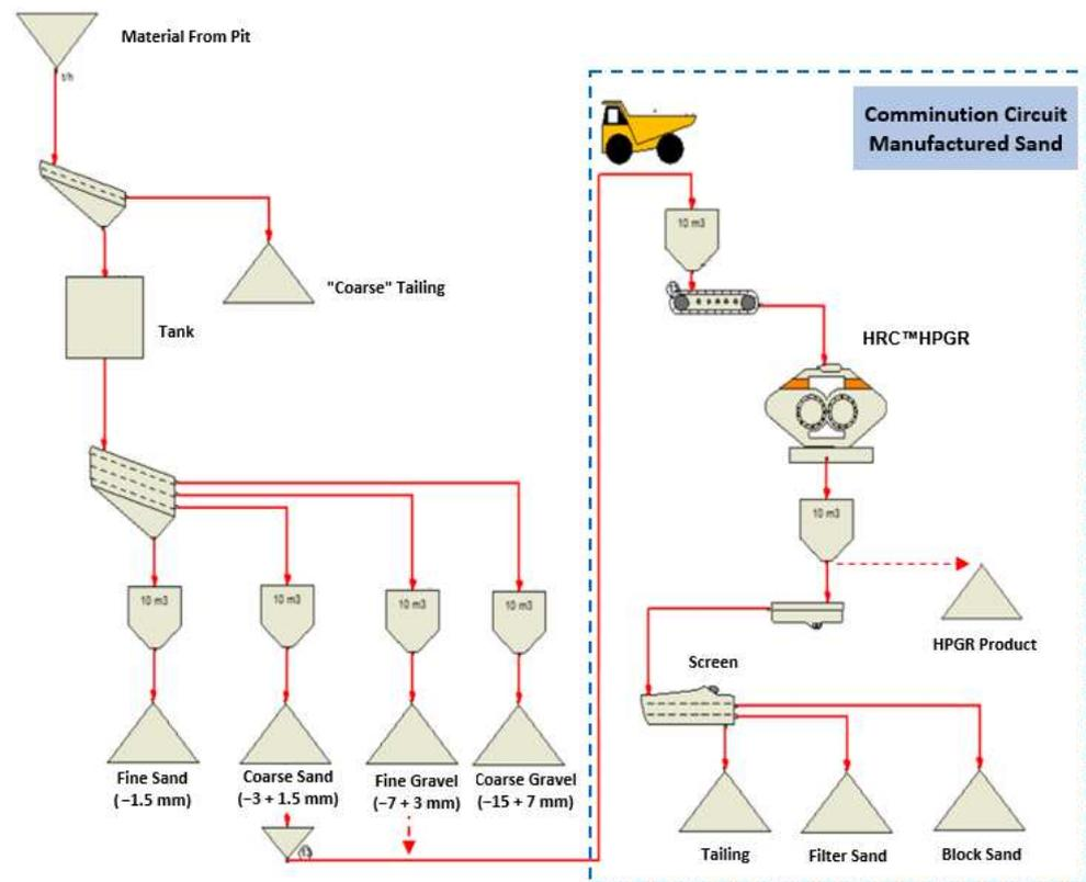
Figure 2. Itaquareia processing plant flow sheet.
