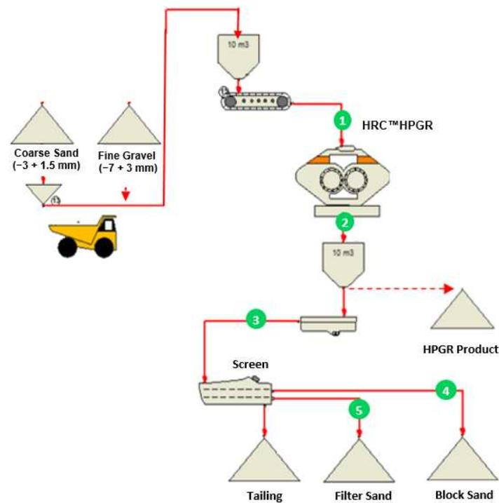
**Figure 5.** Itaquareia comminution circuit and sampled streams.
