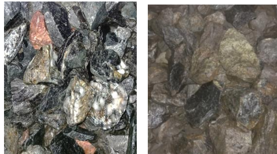
Figure 6 - Left: inclusions recovered with XRT + 3d Laser. Right: material with strong induction signal.
