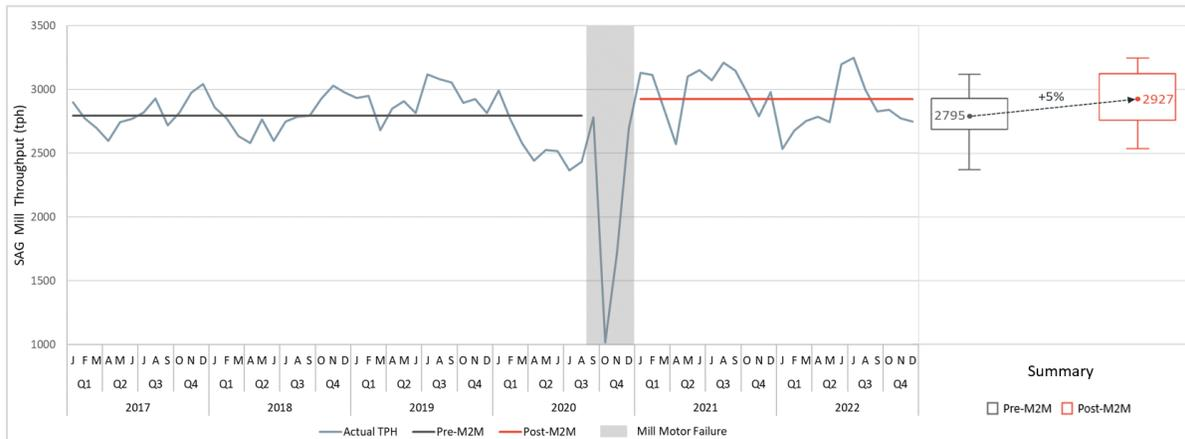
Figure 9—Comparison of Plant Throughput Between Pre- and Post-Mine-to-Mill Periods with Partial Implementation
