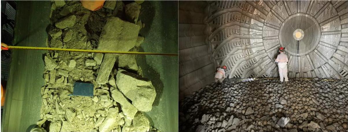
Figure 5—SAG Feed Belt Cut Sampling and Measurements Taken During the SAG Mill Crash-Stop
