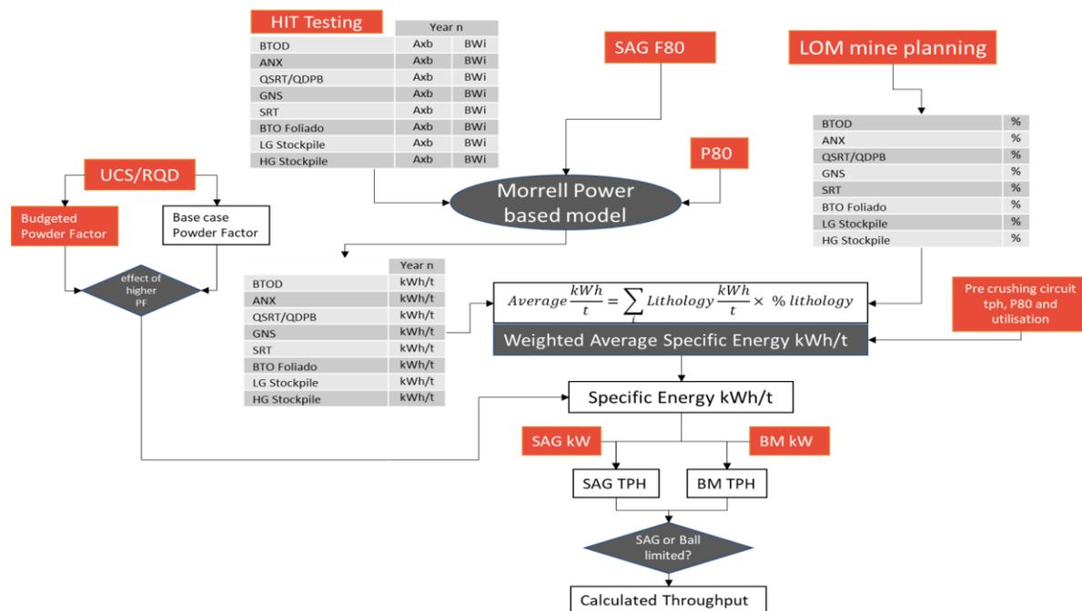
Figure 10—Concept Diagram of the Chapada Throughput Forecast Model
