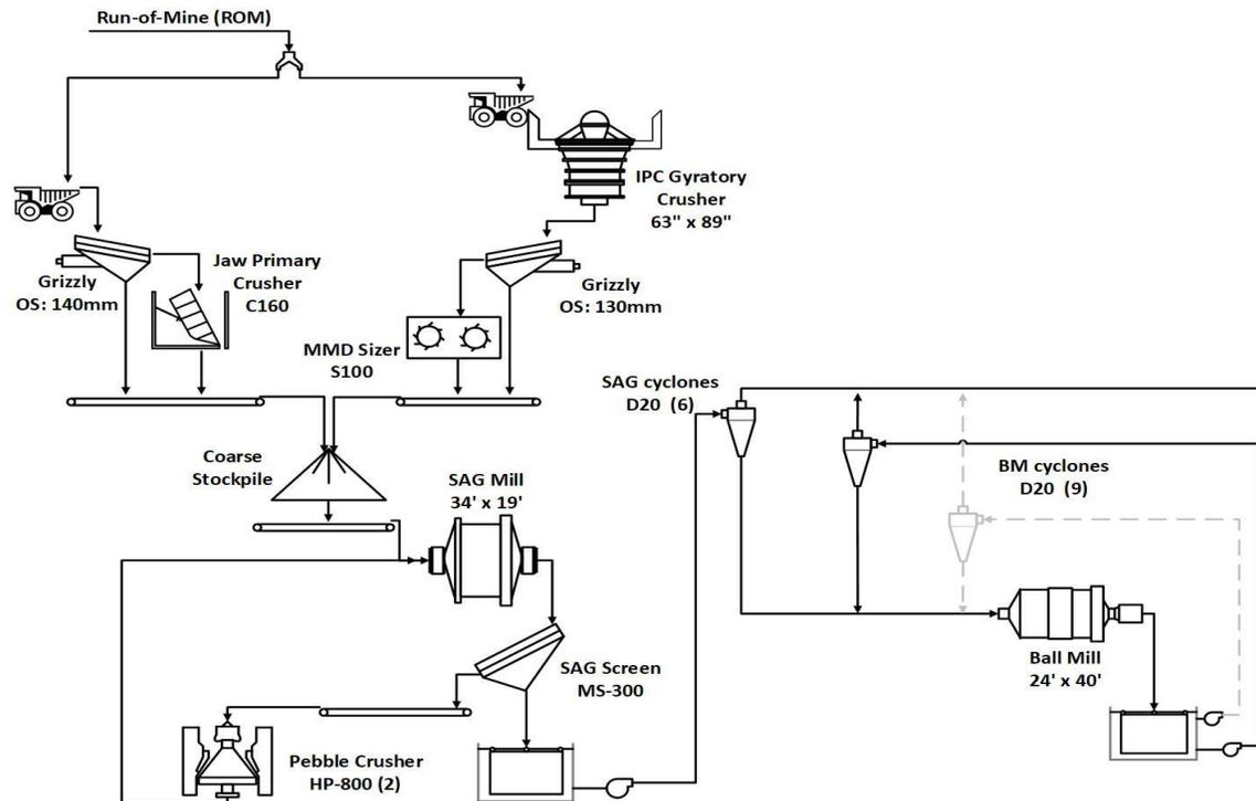
Figure 4—Simplified Flowsheet of the Chapada Comminution Circuit
