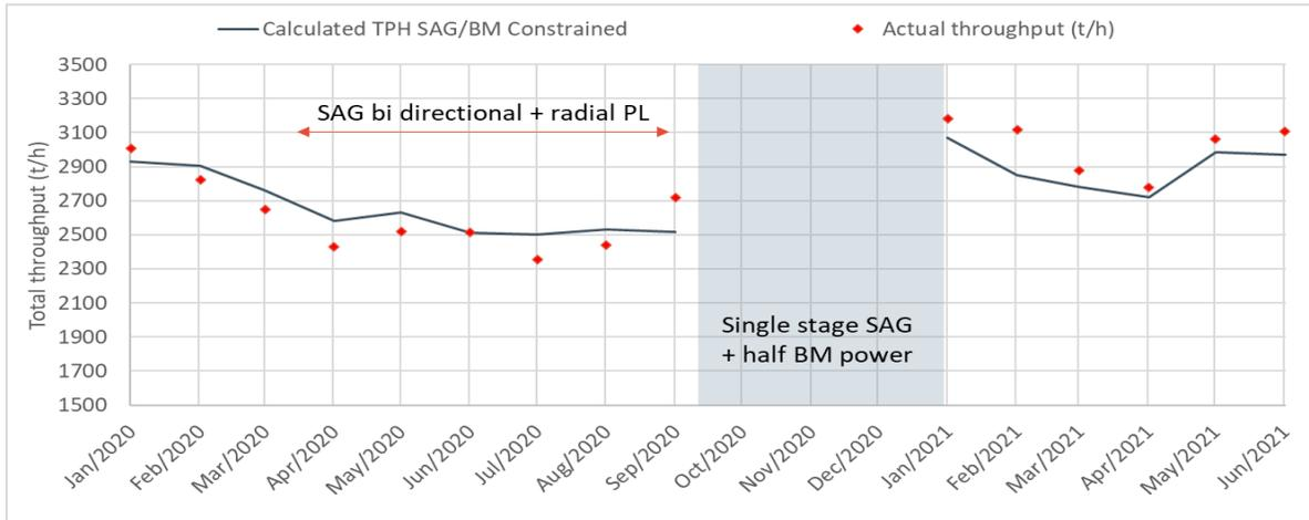
Figure 12—Throughput Forecast Model Validation against Actual Plant Throughput
