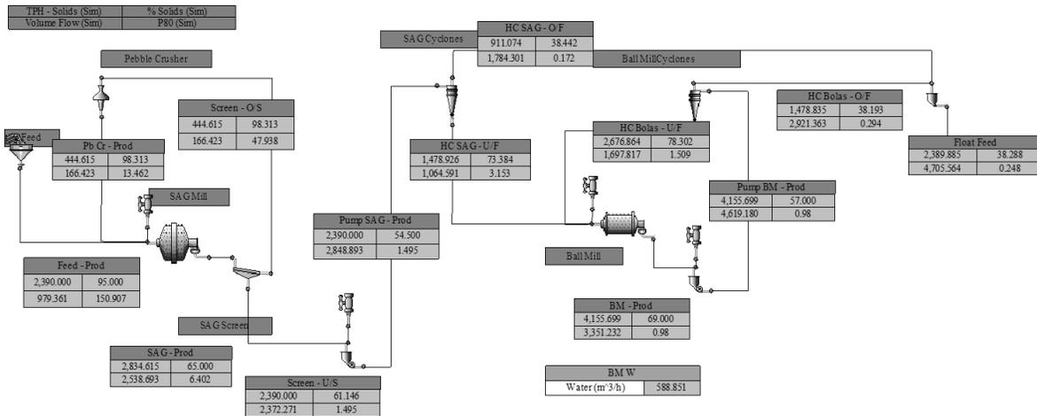
Figure 6—Site-Specific JKSimMet Model of the Chapada Grinding Circuit Model
