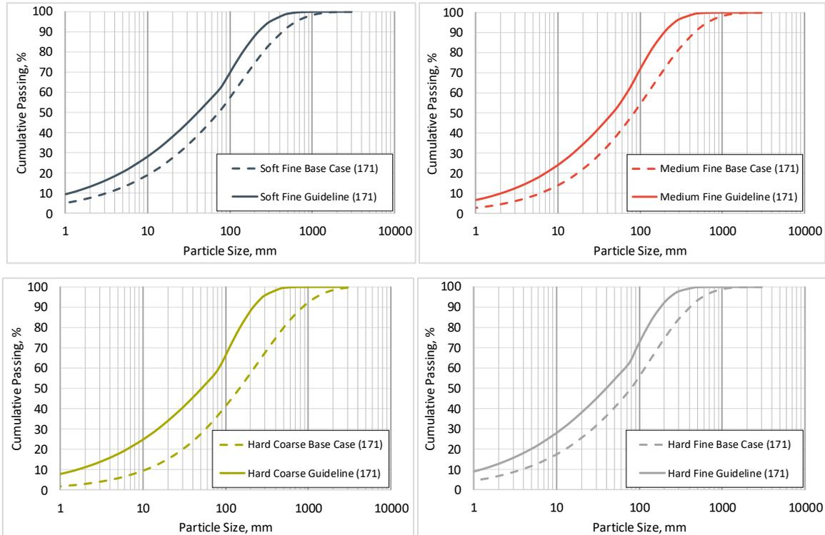
Figure 7—Base Case PSD vs. Optimized PSD from Guidelines for each Ore Domain (Hole Diameter 171 mm)
