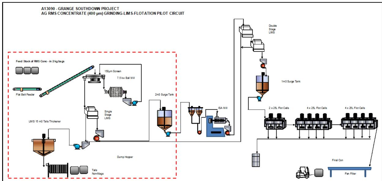
Figure 12: ALS Pilot Ball Milling, Intermediate Magnetic Separation, Regrind Milling and Flotation Flowsheet
