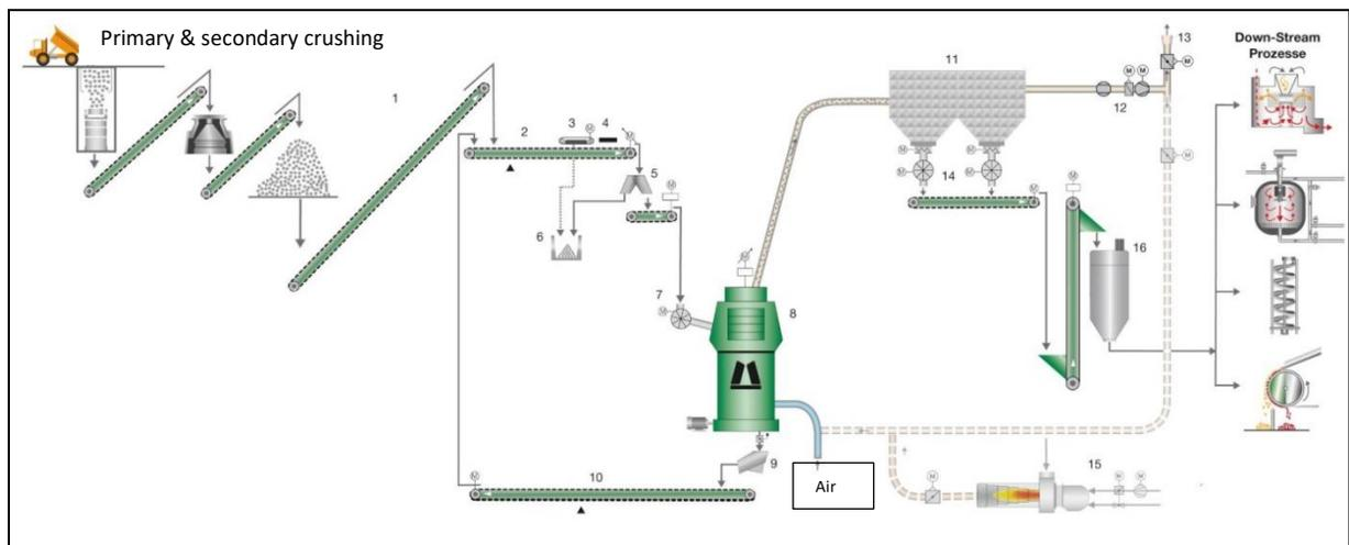
Figure 5: simplified VRM flow sheet with Air Pathways
