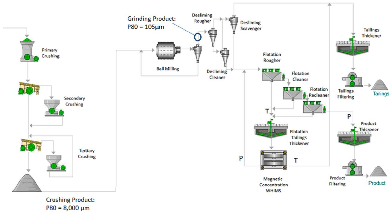
Fig. 1. Conventional itabirite iron ore circuit.
