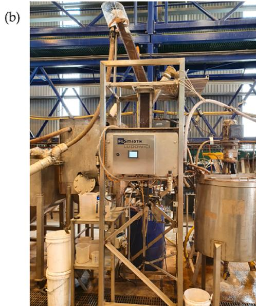
Fig. 6. Schematic representation of the Reflux Classifier (a) and image of the pilot-scale Reflux Classifier (b).
