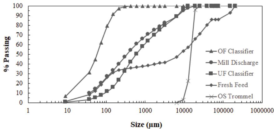
Fig. 9. Size distributions resulting from the pilot-SAG test.
