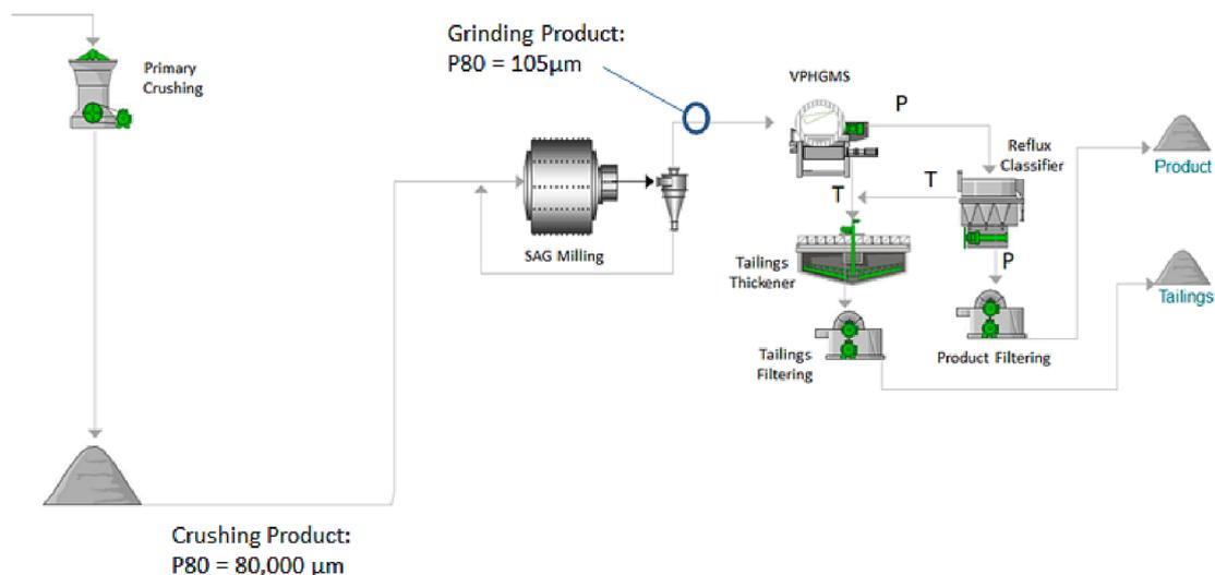
Fig. 2. Proposed disruptive itabirite iron ore circuit.
