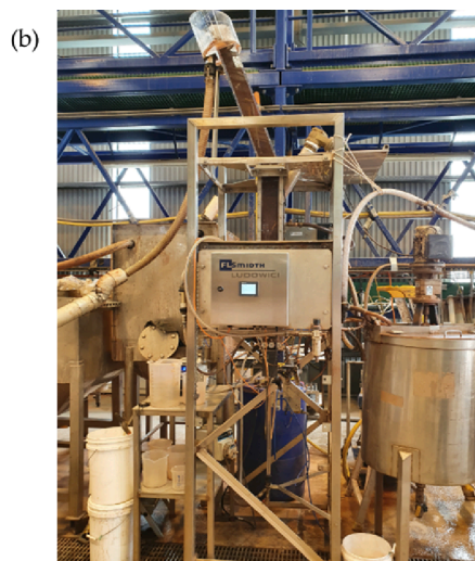
Fig. 4. Reflux Classifier (a) schematic representation (b) image of laboratory system.
