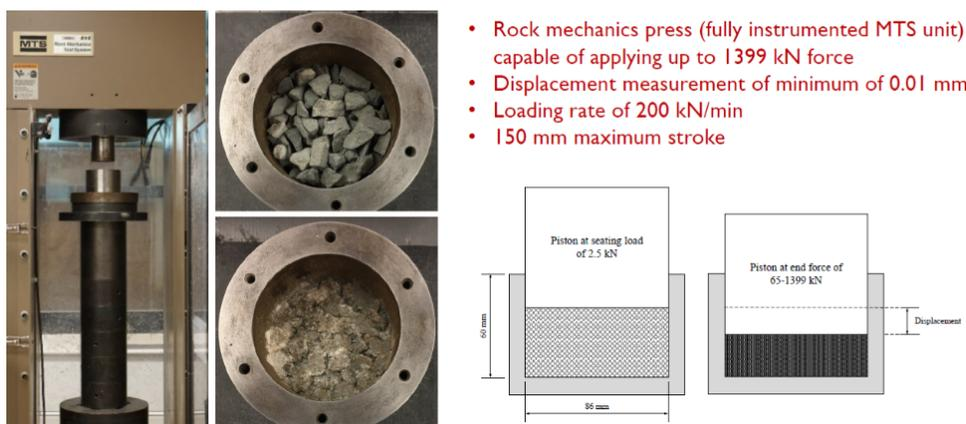
Figure 3a—UBC Piston Press Equipment
