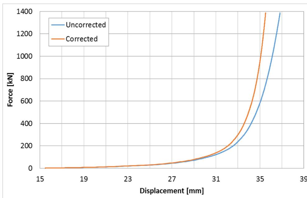
Figure 3b—Example Force-Displacement Curve with Correction for Piston Die Assembly Strain
