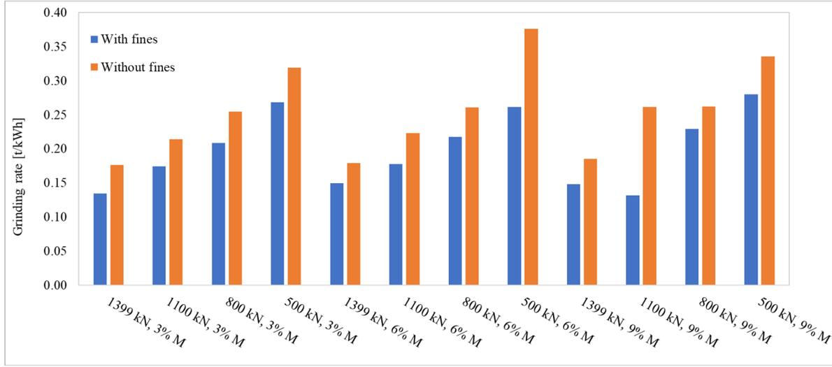
Figure 4a—PGN Ball Mill Feed Sample Piston Press Grinding Rates
