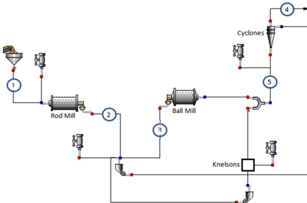
Figure 1—The Porcupine Gold Mine 'A' Grinding Circuit
