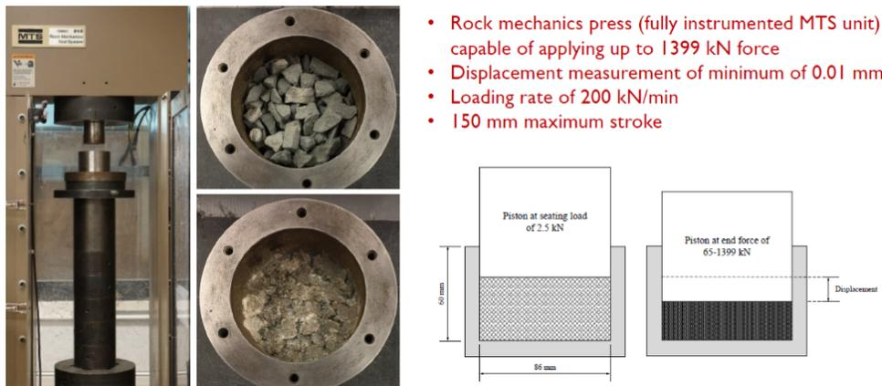
Figure 3a—UBC Piston Press Equipment
