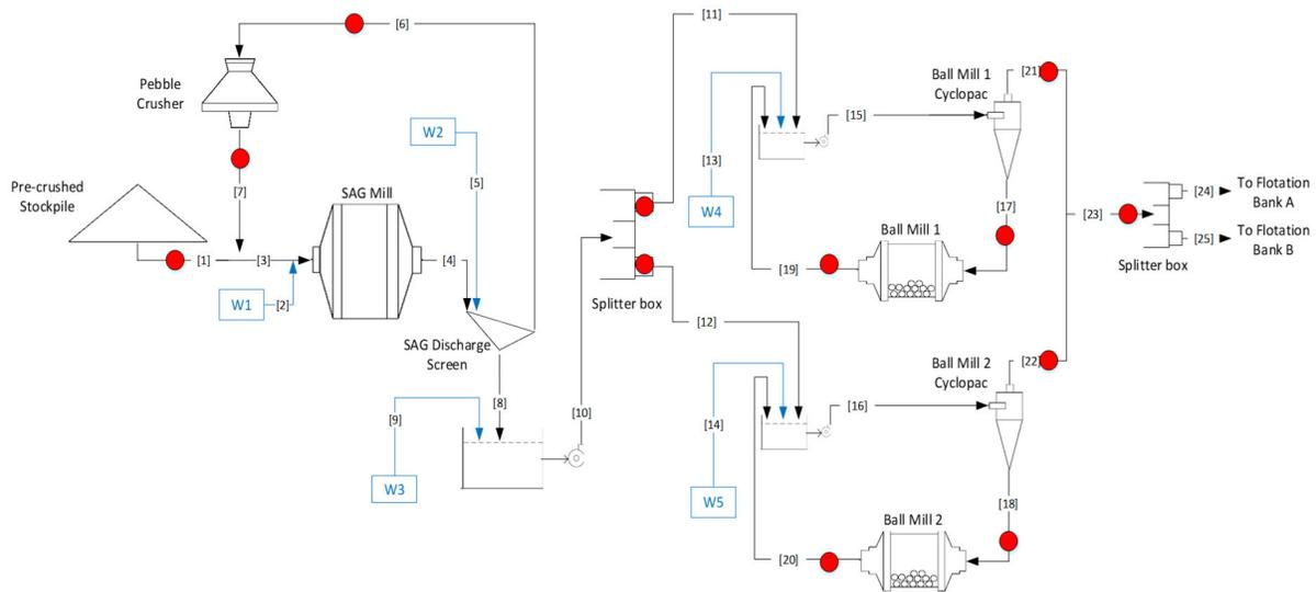
Figure 2—The Copper Mountain Mine Grinding Circuit
