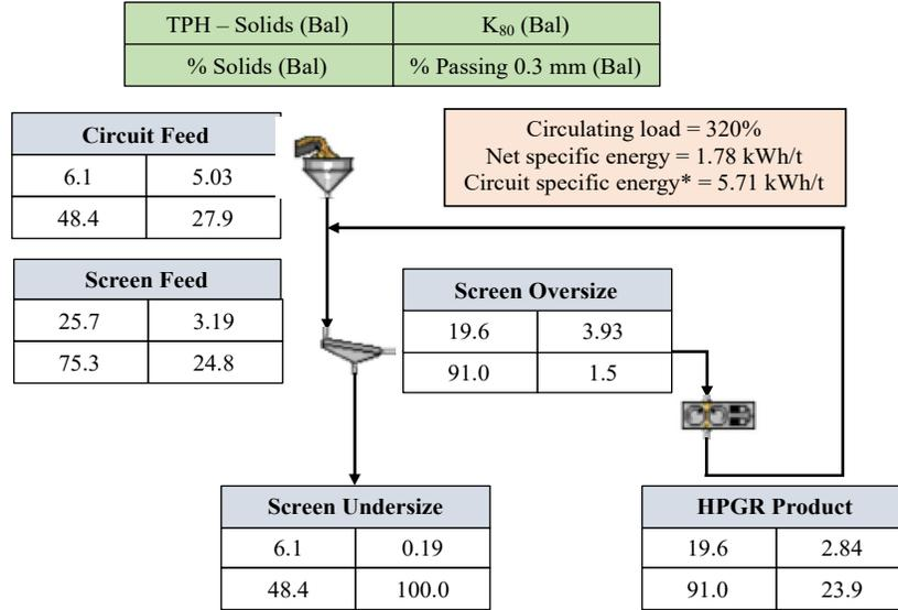
Figure 6—The CMM HPGR Pilot Plant Steady State Conditions
