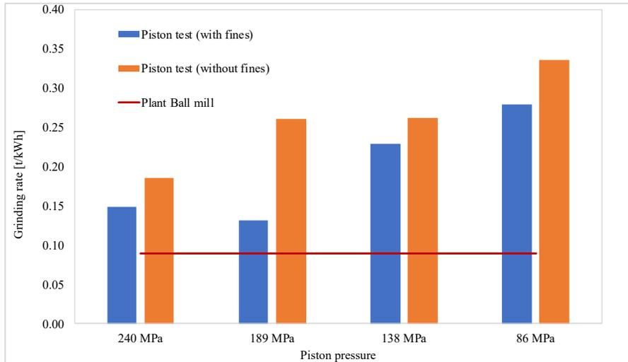
Figure 4b—PGN Mill Feed Sample Piston Press Grinding Rates at 9% Moisture
