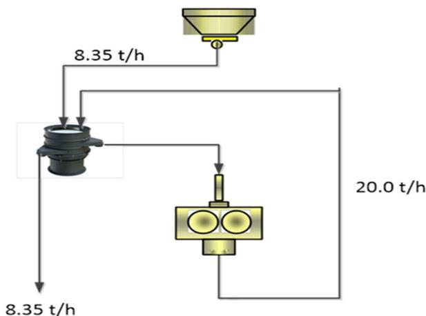
Figure 5—The PGM HPGR Pilot Plant Steady State Conditions
