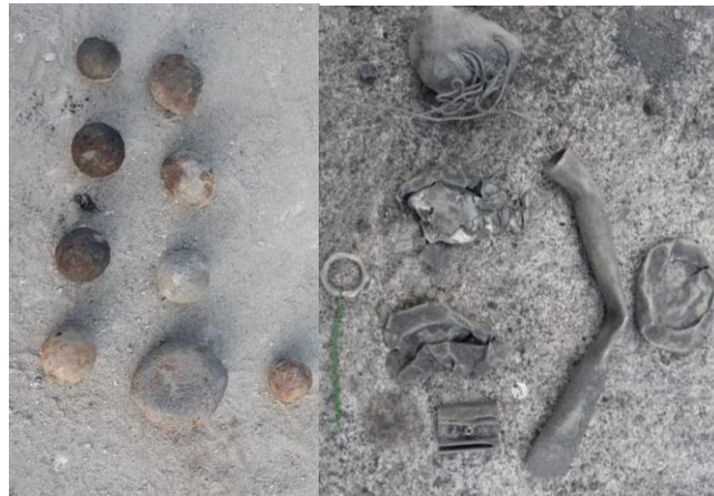
Figure 5: Items in the feed material that were stopped by the metal detector
