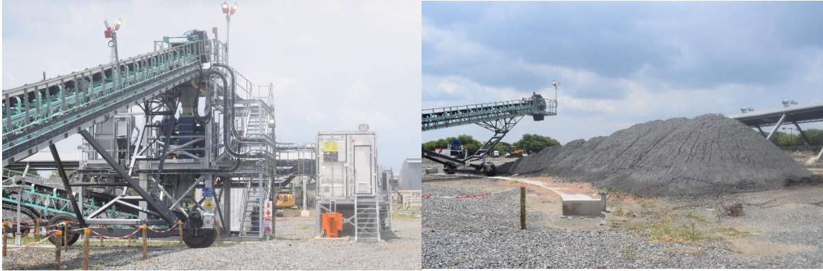
Figure 3: Feed conveyor and EDS Mill (left) and discharge conveyor and kidney stockpile (right)
