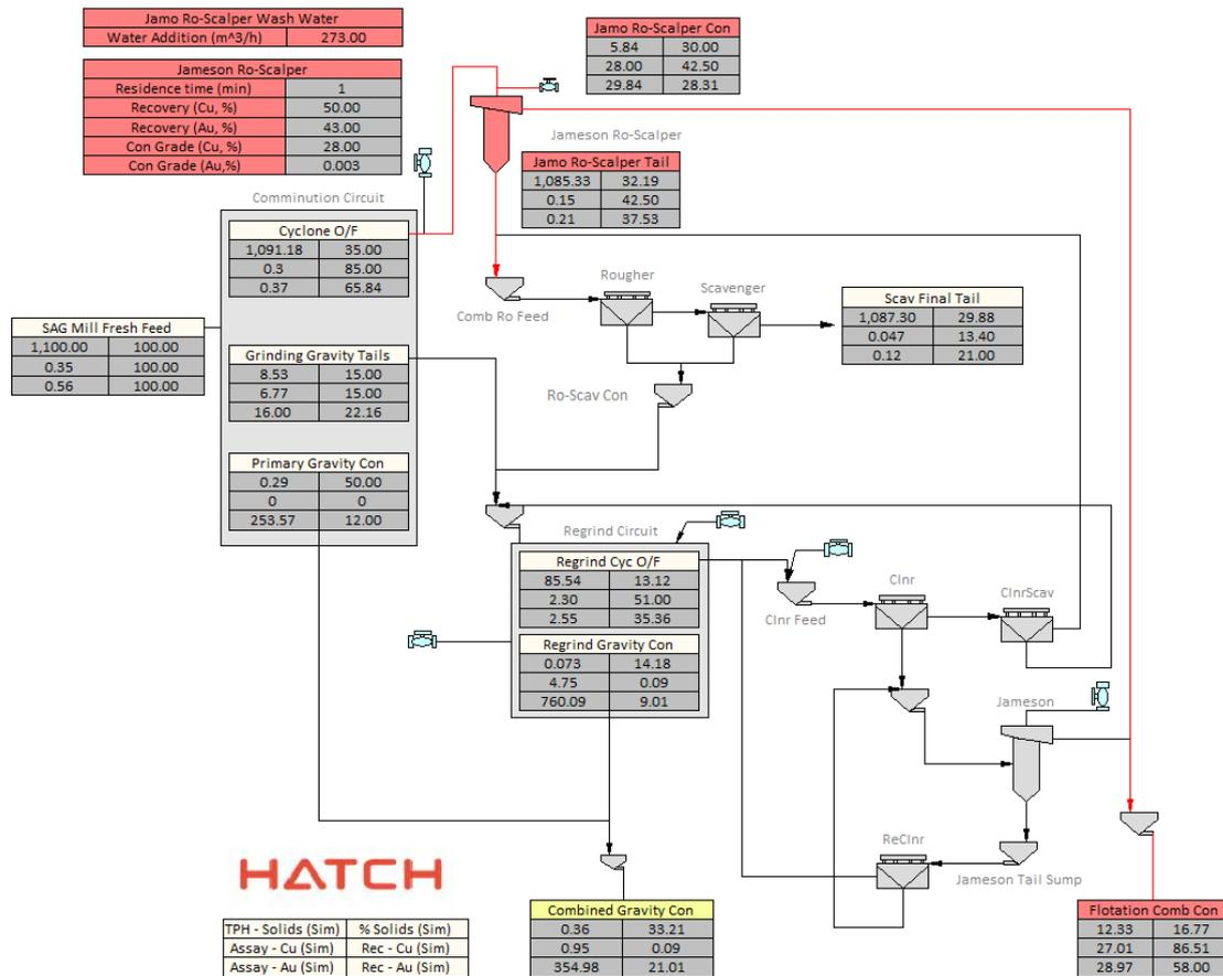
FIG 3 – JKSimFloat model for upgraded flotation circuit with Rougher-Scalper Jameson Cell
