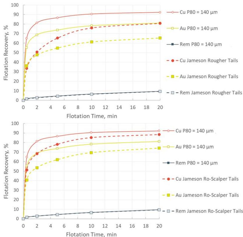
FIG 4 – Cu, Au and Remainder floatability characteristics for flotation circuit feed and Jameson Rougher (top) and Rougher-Scalper (bottom) tails
