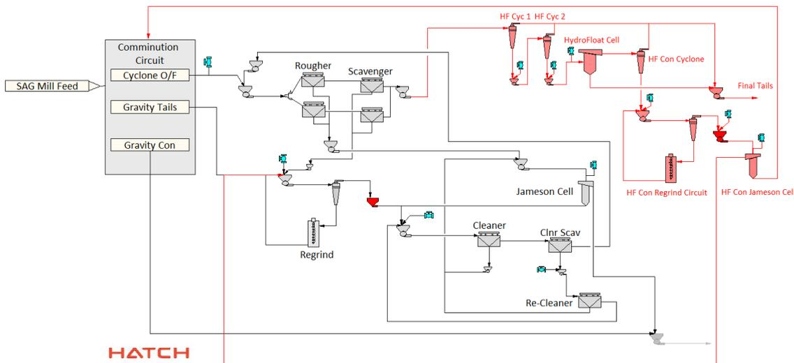
FIG 8 – JKSimFloat model for upgraded flotation circuit with Coarse Particle Flotation Circuit
