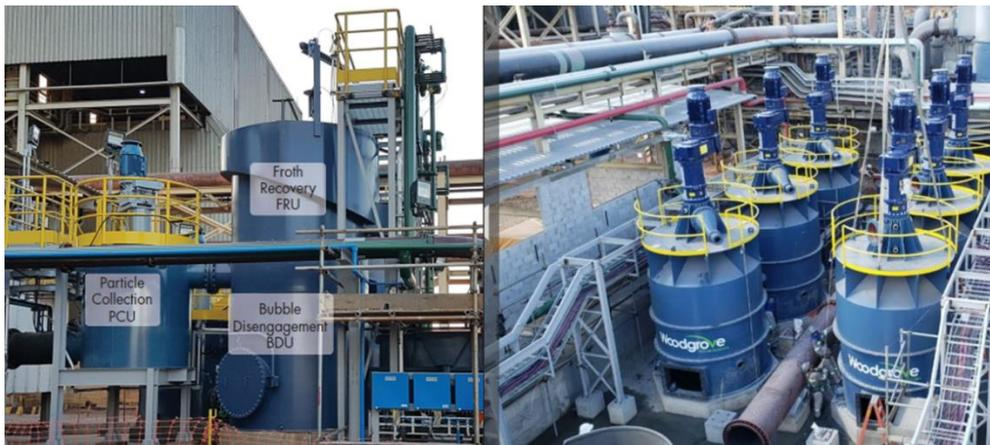
FIG 10 – Woodgrove Staged Flotation Reactor (left) and Direct Flotation Reactors (right) (Nelson and Lelinski, 2019 and Woodgrove Technologies, 2022)
