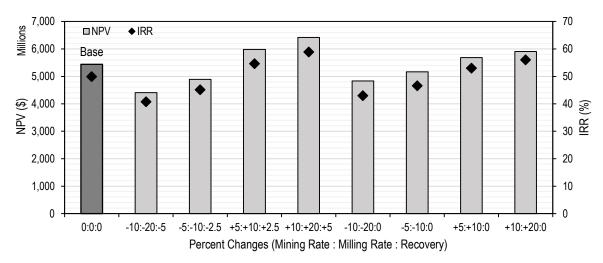
FIG 8 – Results of sensitivity analysis of combinations of key variables by using GEOVIA Whittle™.
