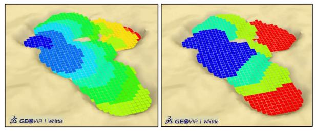
FIG 3 – Pit expansion towards East using directional mining approach (Left) and the four optimal mining phase (pushbacks) selected for scheduling purposes (right) – GEOVIA Whittle™
