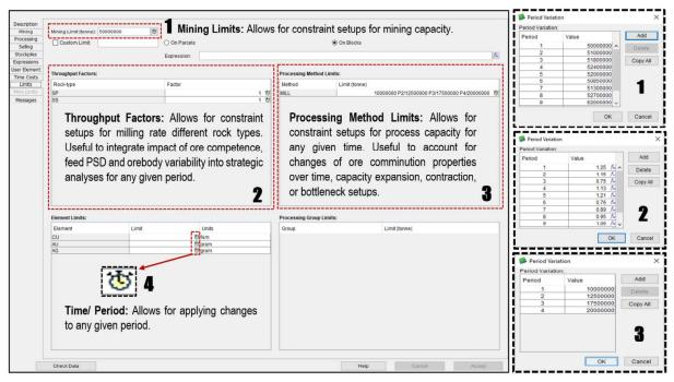
FIG 2 – Mining and processing constraints set-up interface – GEOVIA Whittle™.
